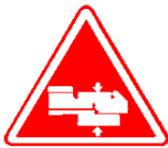
Risk of crushing
