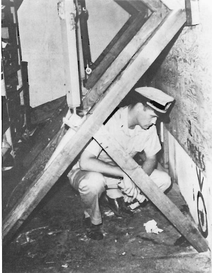
When bulkheads near the flooded compartment threatened to collapse, they were supported by a sturdy complex of timber and steel braces. Ensign John Scott, shown here, supervised the ship's damage control teams.
