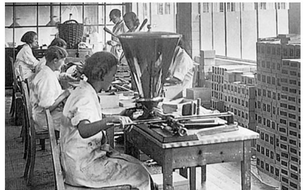
One of the first packing machines in the 1930s was a funnel with an oblong closing mechanism that cut off the flow of tablets when each pack was filled.
