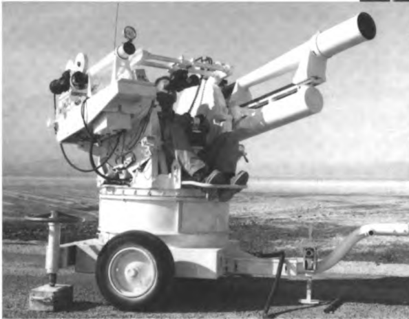
M-45 mobile tracking mount, 1958.
