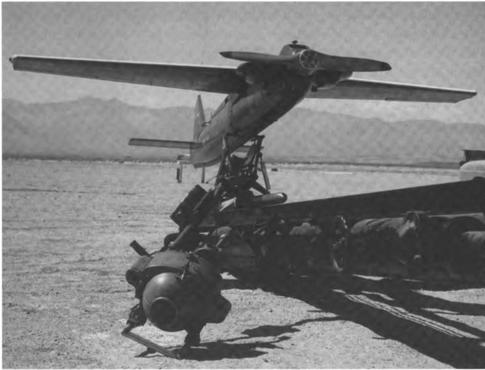
Spot-carrying drone on a compressed-air catapult launcher, April 1954.
