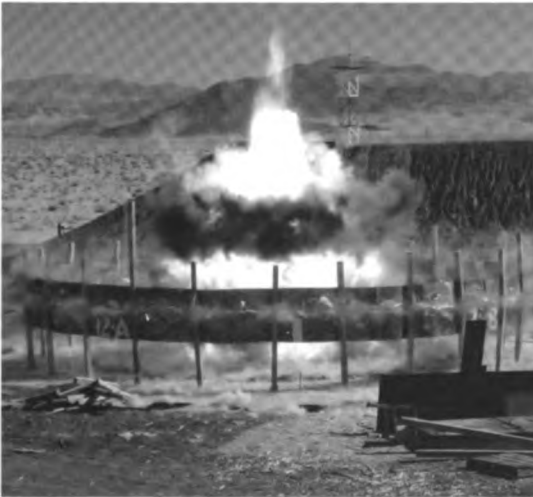
Continuous-rod warhead test at a remote arena. NOTS used the continuous-rod concept in both the Zuni rocket and the Sidewinder missile.
