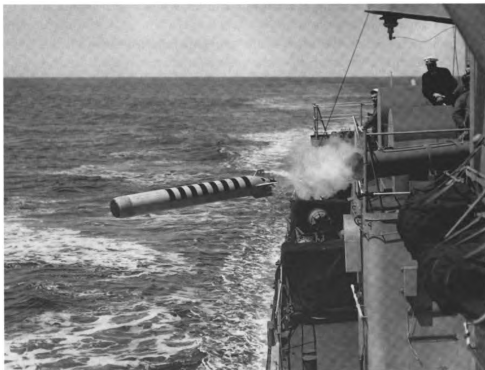
Norfolk (DL-1) launching a Mk 44 Mod 0 lightweight torpedo from the first shipboard ASROC system, 1960.
