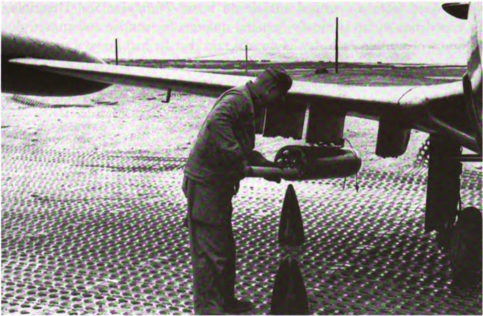
Ordnanceman in Korea loading Mighty Mouse 2.75-inch rocket into NOTS-developed seven-round launcher.
