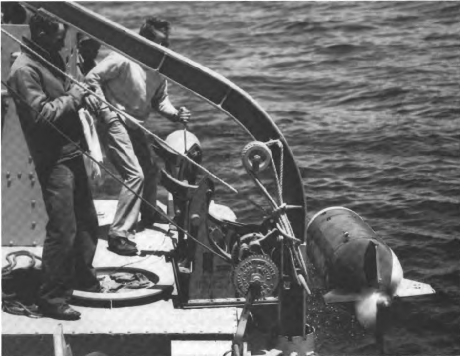
Test at sea of the EX-8 torpedo, later designated Mk 46.
