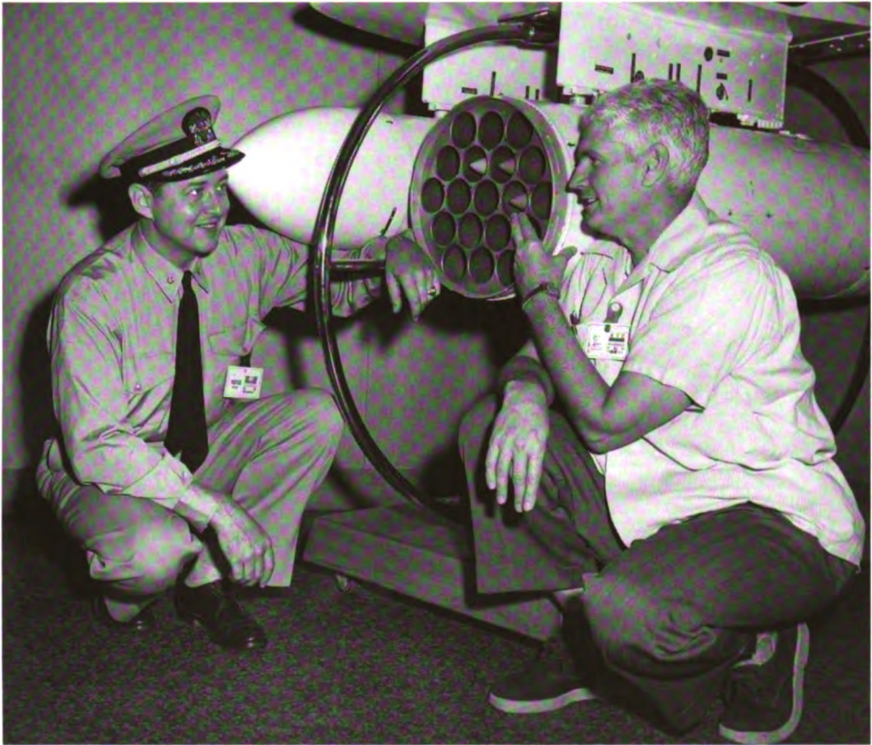
China Lake-developed 19-round disposable rocket launcher.
