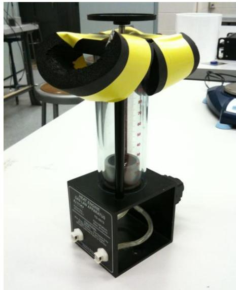
**Note the foam protecting the fragile glass-walled piston; please do not remove this!**
