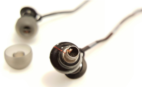
Figure 1 The modified replicator headphone shown modified with a small MEMS microphone attached to monitor and control leakage effects in the listeners' ear.
