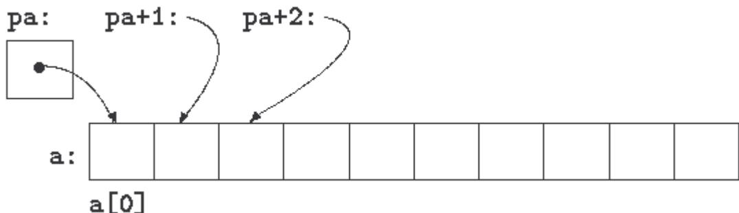
These remarks are true regardless of the type or size of the variables in the array `a`. The meaning of "adding 1 to a pointer," and by extension, all pointer arithmetic, is that `pa+1` points to the next object, and `pa+i` points to the  $i$ -th object beyond `pa`.
