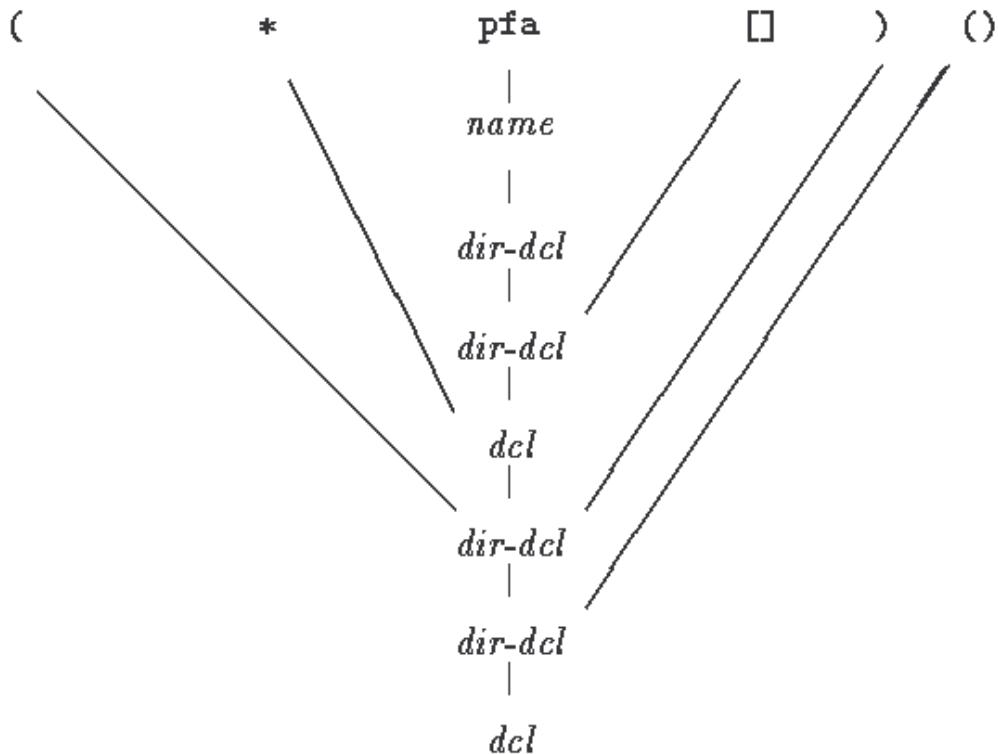
The heart of the `dcl` program is a pair of functions, `dcl` and `dirdcl`, that parse a declaration according to this grammar. Because the grammar is recursively defined, the functions call each other recursively as they recognize pieces of a declaration; the program is called a recursive-descent parser.
