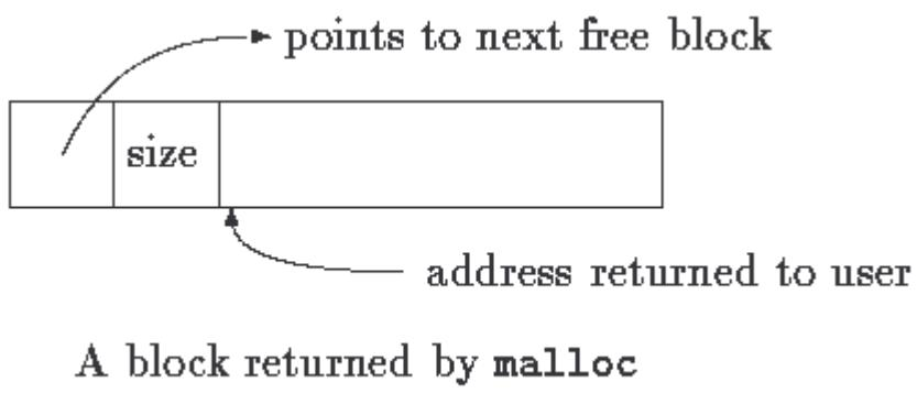
The `size` field is necessary because the blocks controlled by `malloc` need not be contiguous - it is not possible to compute sizes by pointer arithmetic.
