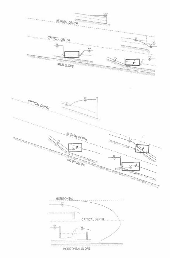
THE CORRECT PROFILES ARE SHOWN IN THE FIGURE ABOVE.
