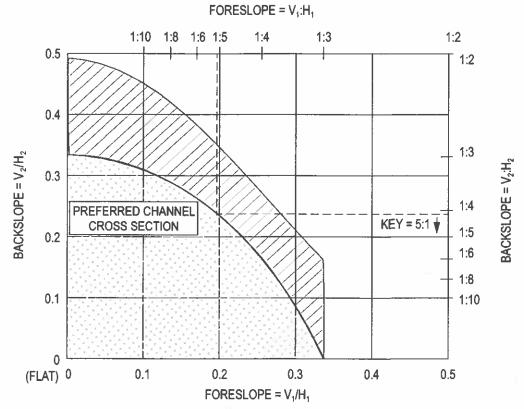
This area is applicable to all Vee ditches, rounded channels with a bottom width less than 2.4 m [8 ft], and trapezoidal channels with bottom widths less than 1.2 m [4 ft].
