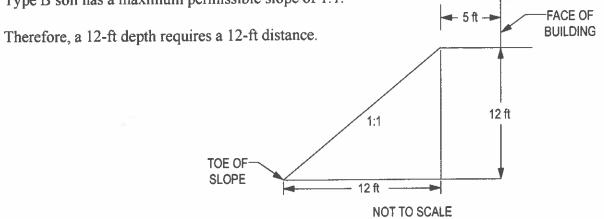
Because there is a 5-ft perimeter strip, the minimum distance from the toe of the slope to the face of the structure = 12 ft + 5 ft = 17 ft.
