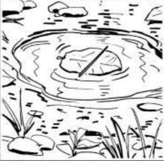
Compass: magnet, needle, straw
