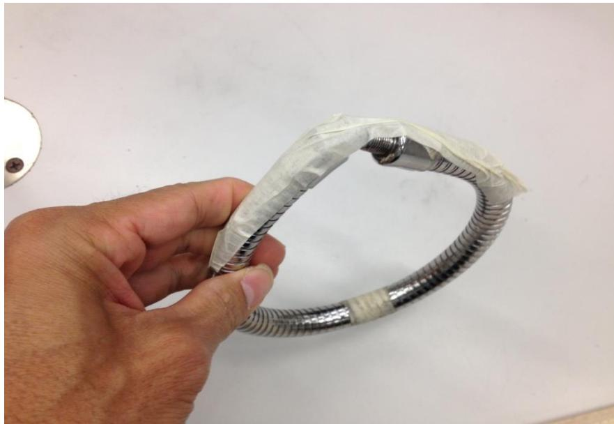
The moment of inertia of circular hoop rotating about an axis perpendicular to and going through its center is:  $I_{(circular\ hoop,\ center)} = mr^2$ . If you cannot bend (and tape) the rod into a perfect circle, you can try either:
