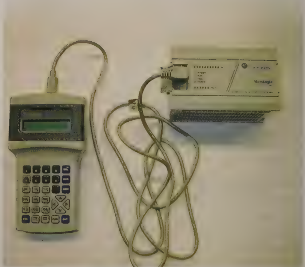
A program can be entered into a programmable controller through a handheld programming device.
