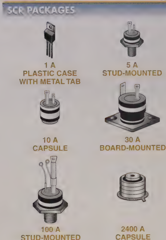
Figure 23-6. SCRs come in a variety of packages, which increase with an increase in current rating.
