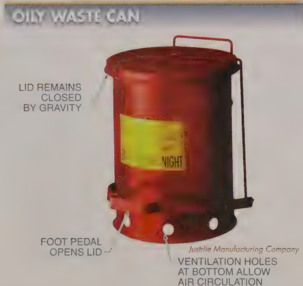
Figure 4-18. An oily waste can seals out oxygen to prevent spontaneous combustion.
