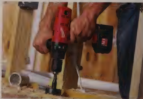
Milwaukee Electric Tool Corporation Cordless hand drills typically contain a brushed DC motor that is powered by a rechargeable battery.
