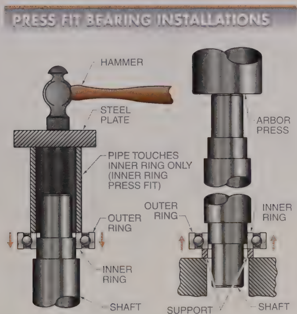
Figure 29-20. During a press-fit installation, uniform force must be applied on the face that is to be press fit using a piece of tubing, a steel plate, and a hammer or using an arbor press.
