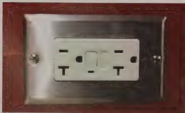
A ground fault circuit interrupter (GFCI) is a device that protects against electrical shock by detecting an imbalance of current in the normal conductor pathways and opening the circuit.
