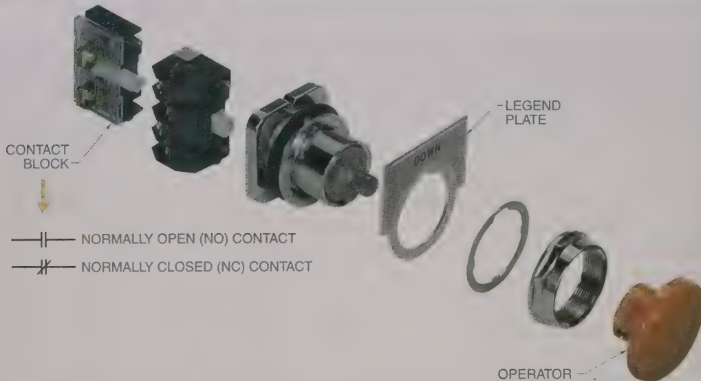
Figure 6-1. An industrial pushbutton consists of a legend plate, an operator, and one or more contact blocks (electrical contacts).
