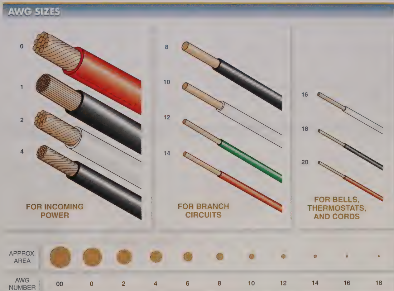
Figure 1-18. The smaller the AWG number, the greater the cross-sectional area and the heavier the wire.
