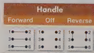
REVERSING DRUM SWITCH INTERNAL SWITCHING
