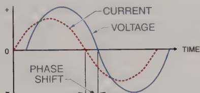
Figure 1-34. Phase shift occurs when voltage and current in an AC circuit do not reach their maximum amplitude and zero level simultaneously.
