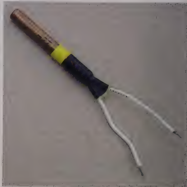
An outdoor air temperature (OAT) sensor is a semiconductor output device used in vehicle and aircraft applications.
