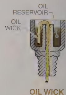
Figure 29-21. Devices used for lubricating bearings include grease fittings, pressure cups, oil cups, and oil wicks.
