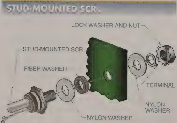
Figure 23-13. SCRs, like regular silicon diodes, can be stud-mounted.
