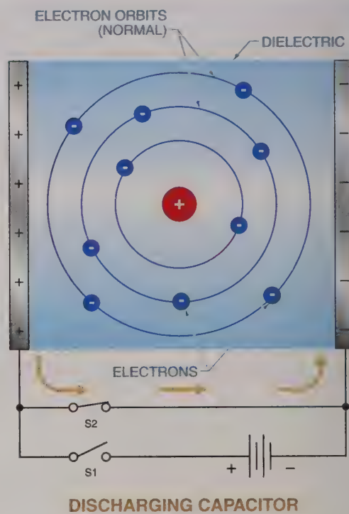
Figure 1-36. With a charged capacitor, the electron orbits become stretched toward the positively charged plate.
