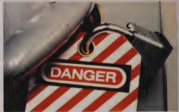
Figure 4-7. Equipment must be locked out and/or tagged out before installation, preventive maintenance, or servicing is performed.
