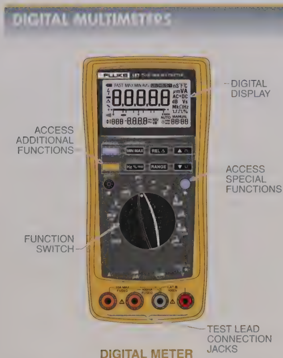
Figure 3-11. Digital multimeters use an LCD to show electrical measurements.
