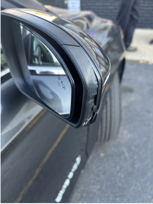
13 | Inspection photo Exterior mirror housing with cracking visible.
