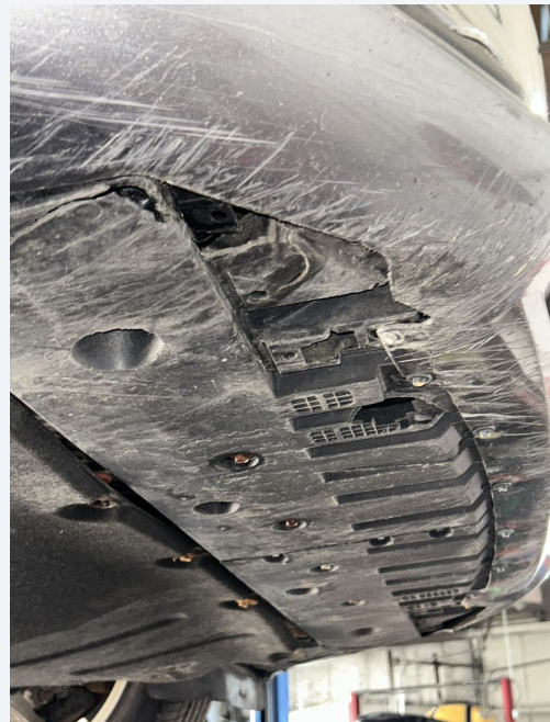
12 | Inspection photo Damaged/scuffed lower undertray.
