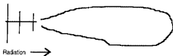
Figure 50. A directional antenna pattern.
