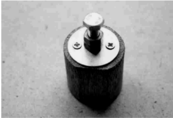
The finished seating die.
