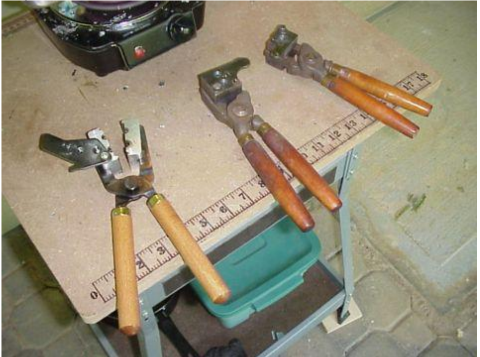
A Lee double cavity mold on the left show with its sprue open, and two Lyman molds, a double and a single.
