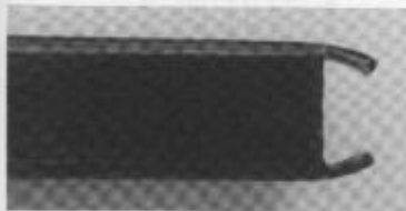
PHOTO 48: Magazine lips after forming.
