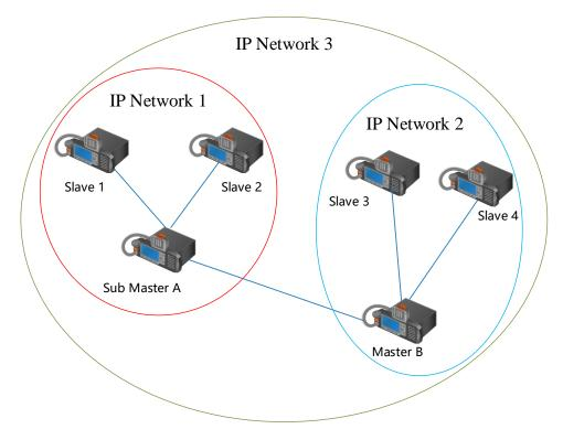
In IP Transit network, portable radio and mobile radio support full services of digital functions in Direct mode, including voice, data and signaling. To get a more detailed list of radio features, please refer to *New Generation DMR Radio\_Feature List*.
