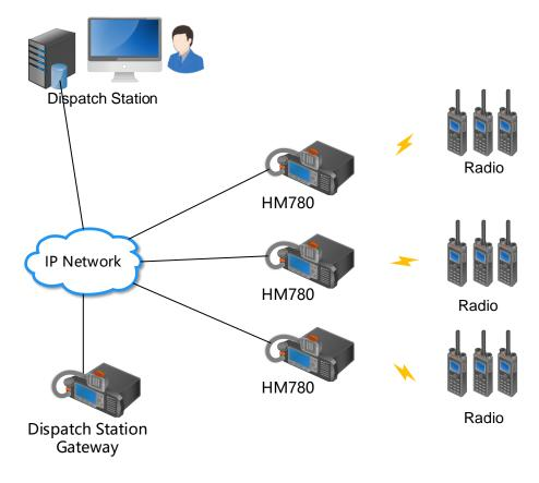
The following is a typical network diagram for developing a scheduling system based on IP network port.
