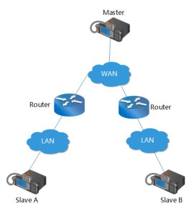
As shown in the figure above, the slave mobile radio A and slave mobile radio B locate in different LANs, which have different network addresses. In this case, the slave mobile radio must have an Ethernet IP address for port mapping via the router, so as to connect to the master mobile radio and other slave mobile radios. Please refer to the appropriate router manual for details.
