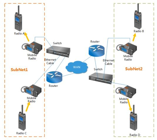
mobile radio, which is responsible for connecting multiple mobile radios in different subnet to realize IP Transit network.
