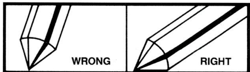
Figure E: Correct and incorrect way to hold the soldering iron against the parts to be soldered.
