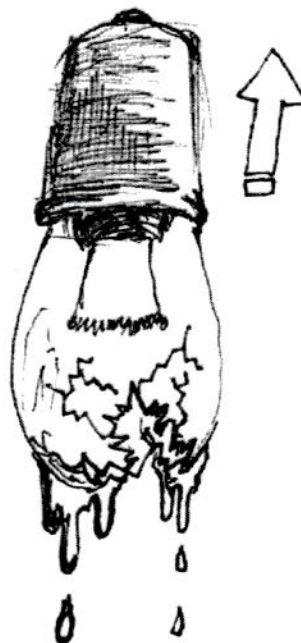
Figure R: Remove the bulb, being careful not to let any water touch the filament.
