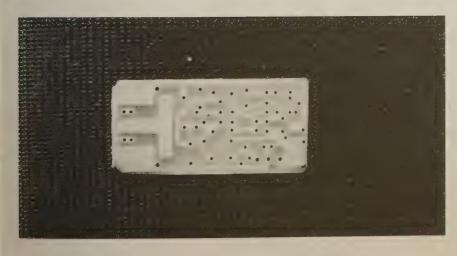
SXC-48/49 combo PCB. Here is the SXC-49 PCB etched, tinned, and drilled. The image is about 10 percent larger than actual size. This PCB can be used for the SXC-49 room bug or the SXC-48 phone tap.
