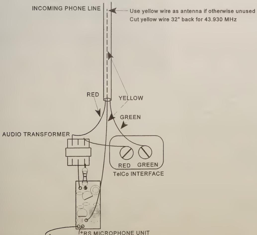
Figure 4. Use this diagram to assist in covertly planting the Radio Shack microphone in a standard TelCo interface.
