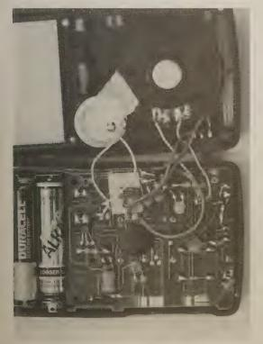
Tone Dialer rewiring. Note the location of new SPDT switch and routing of wires. You only need to clip the left leg of the ceramic resonator. There's no need to remove it.
