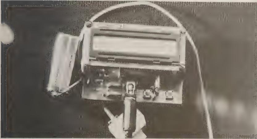
For best results, the decoder module and LCD readout module should be built onto a single PCB. With a little care and patience, you will have a professional-looking finished product!
