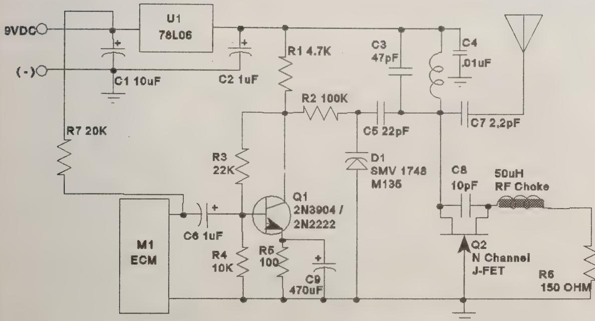
Figure 6. Schematic diagram for the SXC-49 FET-driven oscillator.
