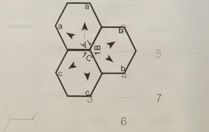
Figure 32. Antenna placement can be thought of in two ways. The antenna tower can be thought of as being at the cell center radiating waves in three directions, as represented by the dotted hexagons, or you can think of it as three separate antenna towers placed at the cells' opposite corners. The lowercase letters represent the opposite-corner towers in the solid hexagons.
