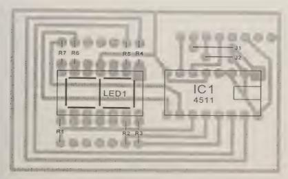
Figure 25. Stuffing diagram for seven-segment readout module
