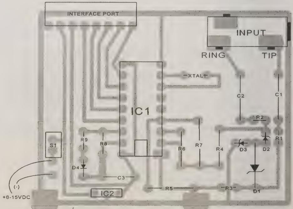
Figure 18. Stuffing diagram for decoder module.
