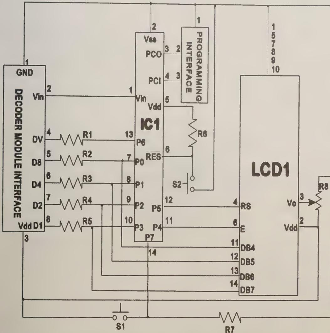
Figure 26. Schematic for LCD readout module.
