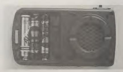
Placement of crystal. Due to lack of real estate, the new crystal must be hidden in the battery compartment. Battery compartment cover operates normally with crystal in place.
