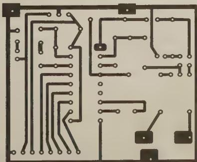
Figure 17. Foil pattern for decoder module.
