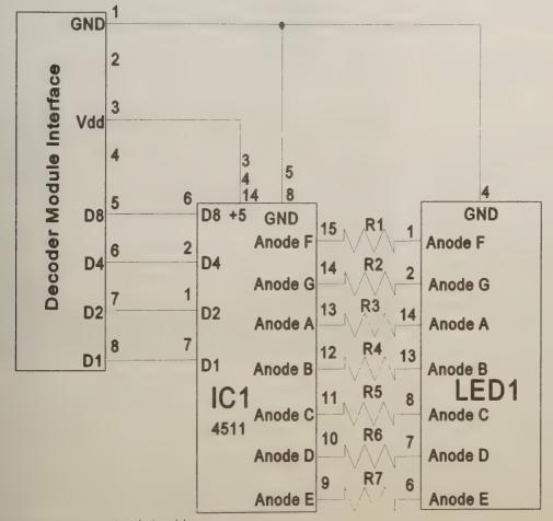
Figure 23. Schematic for seven-segment readout module.
