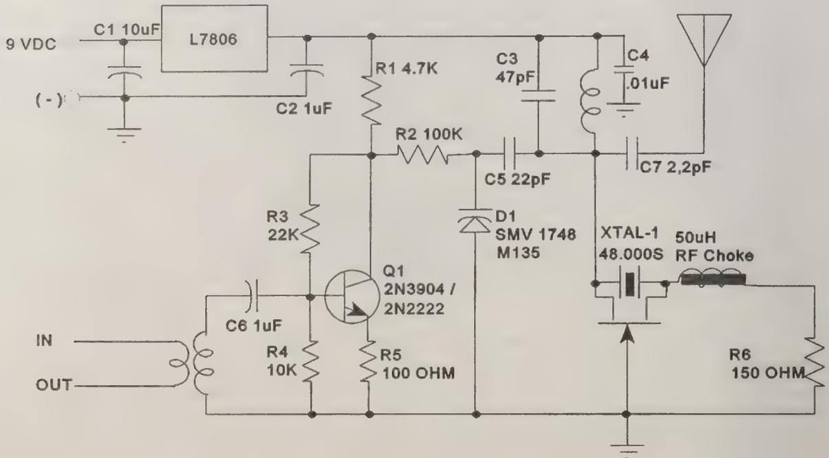
Figure 9. Schematic diagram for the SXC-48.
