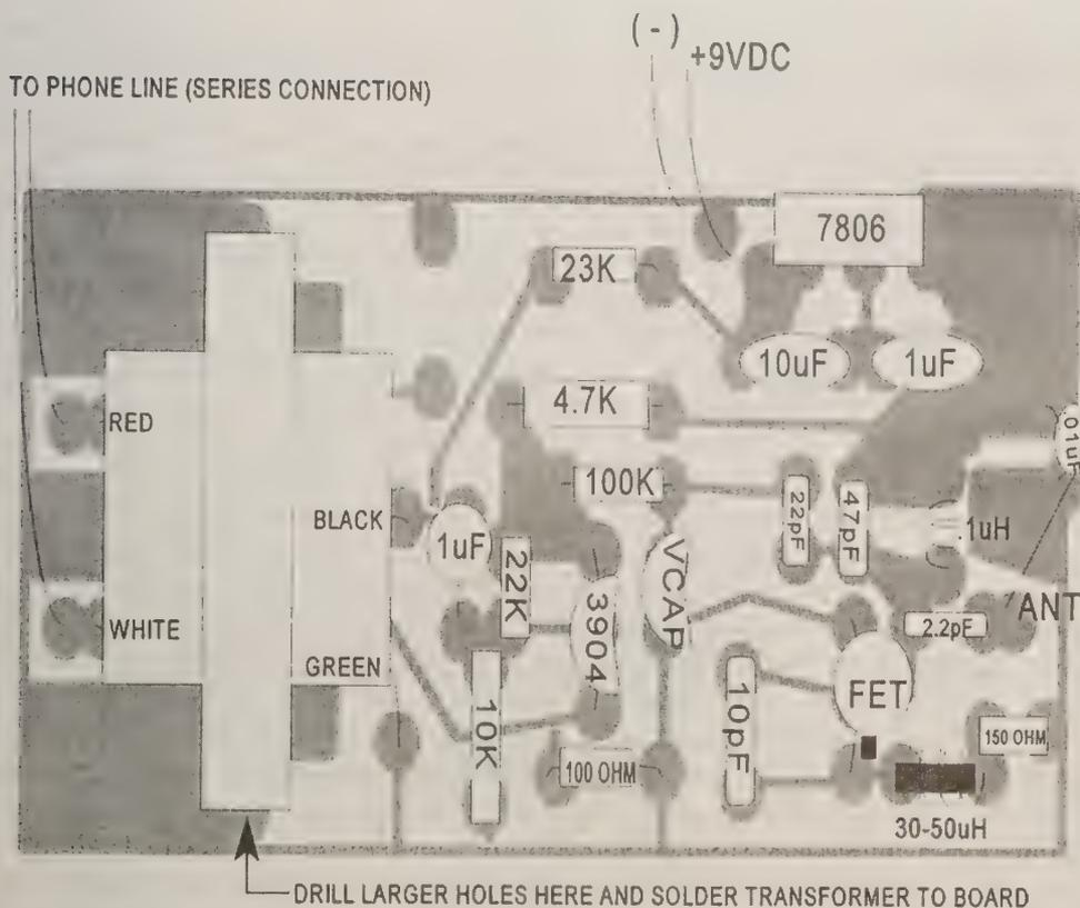
Figure 11. Stuffing diagram for the SXC-48.
