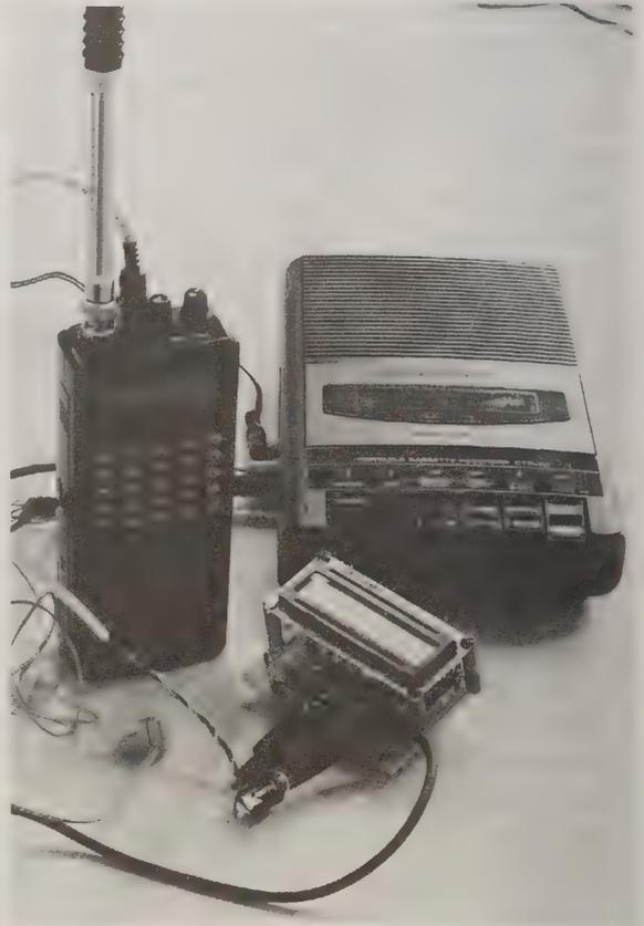
Decoder module prototype with LCD readout (built on a single board) hooked up to a scanner and Radio Shack tape recorder. Output from the scanner is taken from the headphone jack through a homemade "Y" adapter. Output from the "Y" adapter is fed into the decoder module input jack and the AUX INPUT jack of a tape recorder. Earphone output is taken from the recorder. To do this, the recorder must be placed in record mode. Keep the tape paused until something exciting happens!
