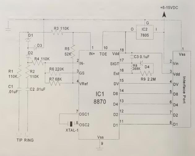
Figure 16. Schematic for decoder module.
