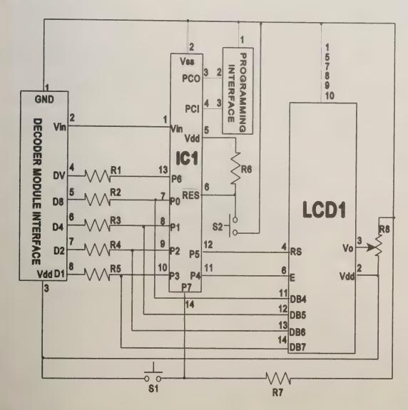
Figure 26. Schematic for LCD readout module.
