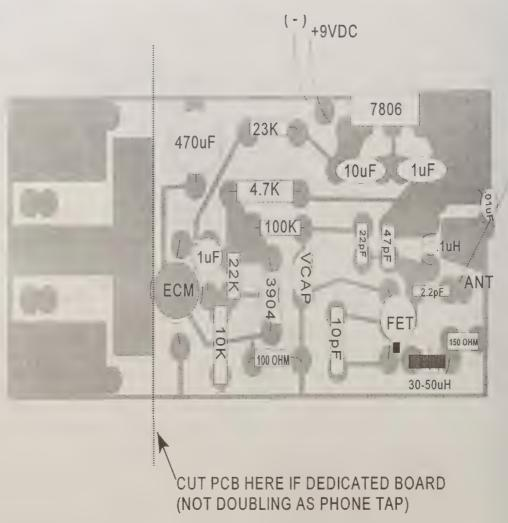
Figure 8. Stuffing diagram for the SXC-49.
