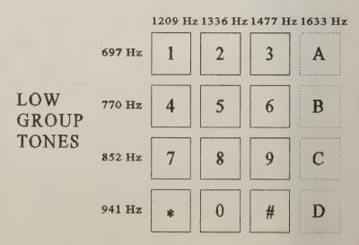
Figure 13. As its name suggests, a DTMF tone is composed of two tones. One tone is taken from the high group, and the second tone is taken from the low group. Use this chart if you ever desire to know which two frequencies make up a particular DTMF tone. For example, the digit 5 is composed of 1,336 Hz and 770 Hz.
