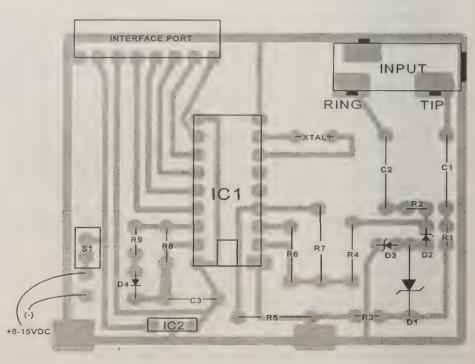
Figure 18. Stuffing diagram for decoder module.
