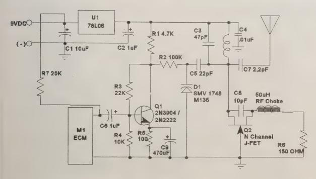
Figure 6. Schematic diagram for the SXC-49 FET-driven oscillator.
