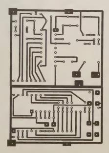
Figure 27. "Combo-board." If you've come this far, you might as well burn the whole board. If you only need the foil pattern for the LCD readout module, cut at the arrows and use the side marked "LCD." The extra solder pads at pins 2 and 6 of IC1 are from an older version and are not used in this project. Use a 1/32-inch drill bit or small Dremel bit to drill the holes.
