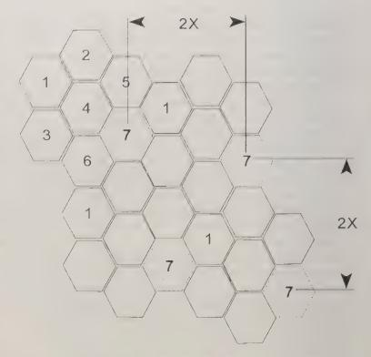
Figure 30. Typical cell block arrangement for seven-cell layout.
