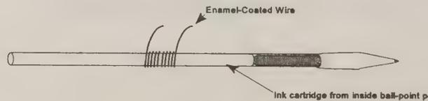
Figure 5. L2 can be made by wrapping about 20 turns of enamel-coated wire around a ferrite core. The prototype, however, used a 33  $\mu$ H molded choke.
