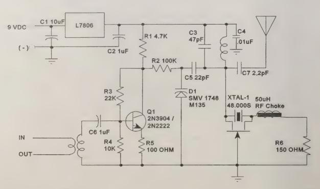
Figure 9. Schematic diagram for the SXC-48.
