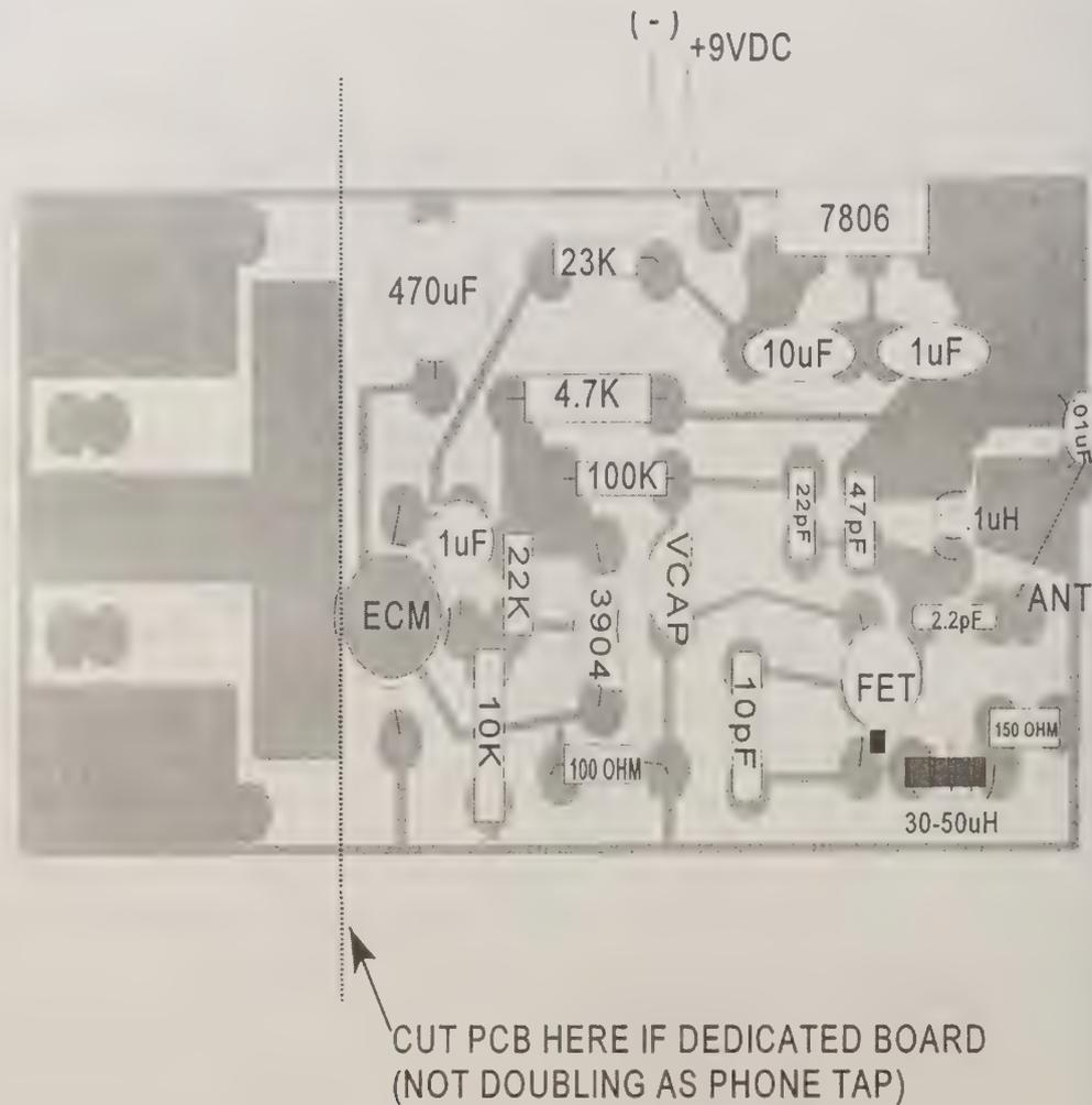
Figure 8. Stuffing diagram for the SXC-49.
