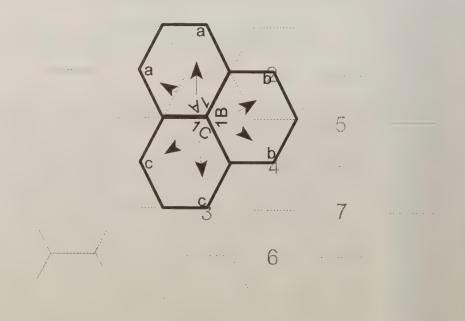
Figure 32. Antenna placement can be thought of in two ways. The antenna tower can be thought of as being at the cell center radiating waves in three directions, as represented by the dotted hexagons, or you can think of it as three separate antenna towers placed at the cells' opposite corners. The lowercase letters represent the opposite-corner towers in the solid hexagons.
