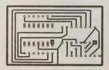
Figure 24. Foil pattern for seven-segment readout module.
