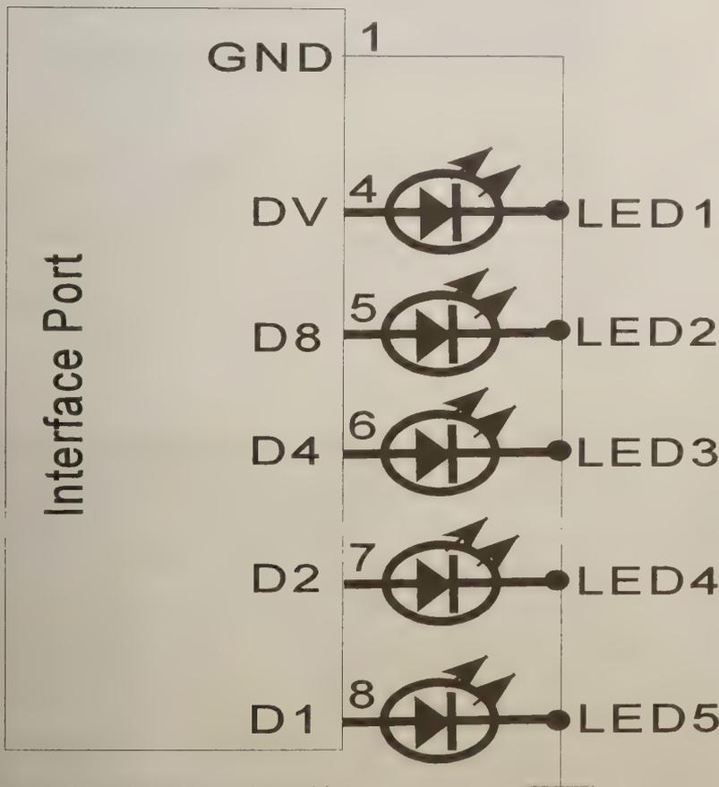
Figure 20. Schematic for binary readout module.
