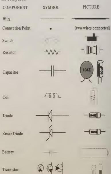
Figure 2. This chart is a quick reference for the schematic symbols used in the coming projects.
