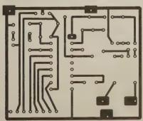
Figure 17. Foil pattern for decoder module.
