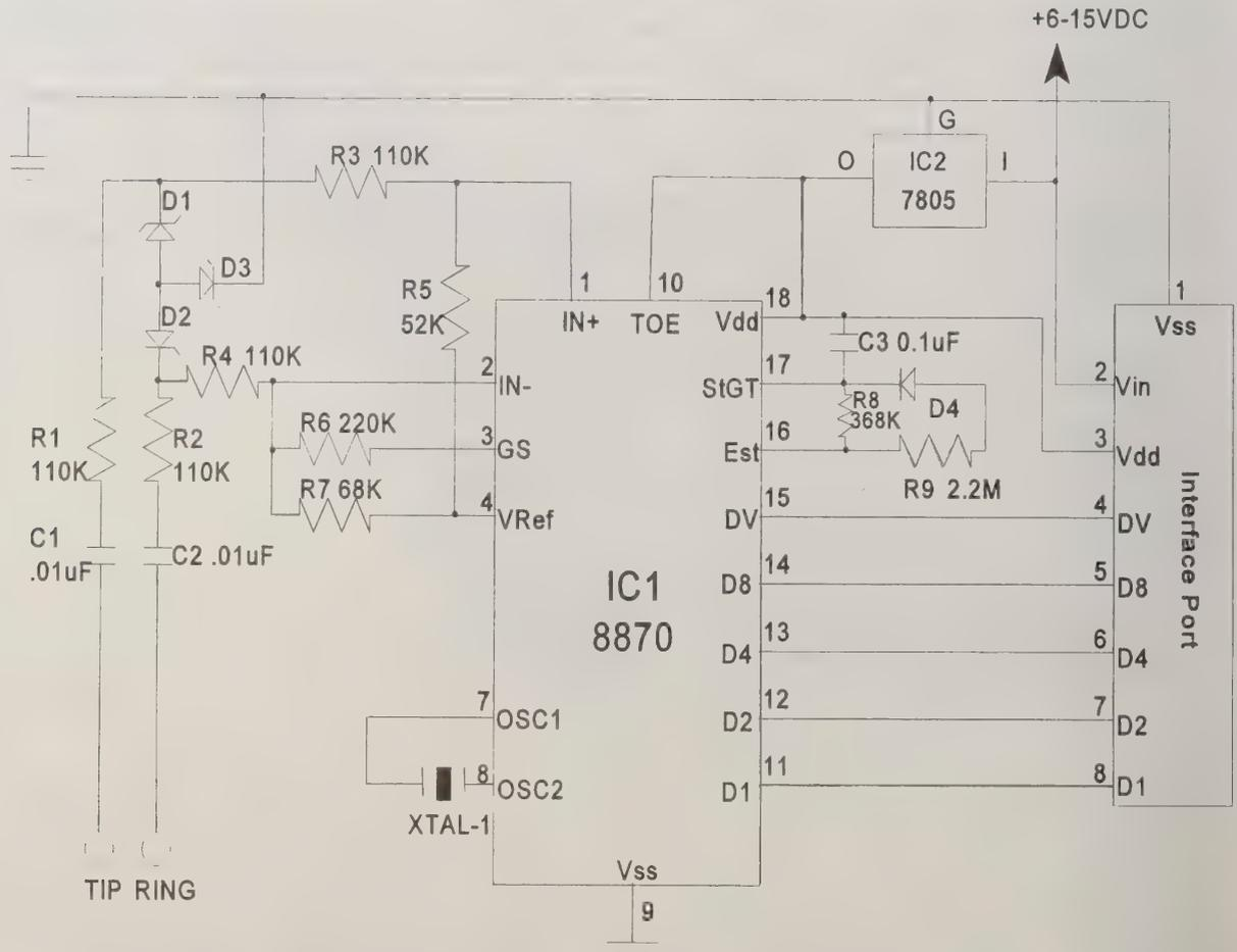
Figure 16. Schematic for decoder module.
