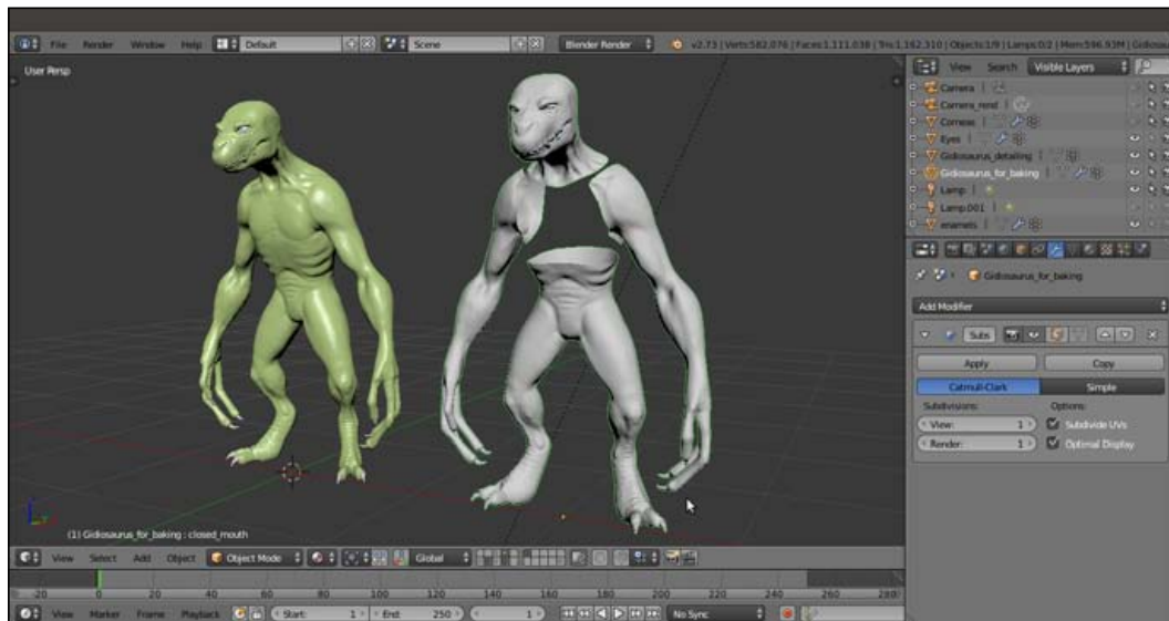
Comparison between the high resolution sculpted mesh and the low resolution object with the baked normal map
