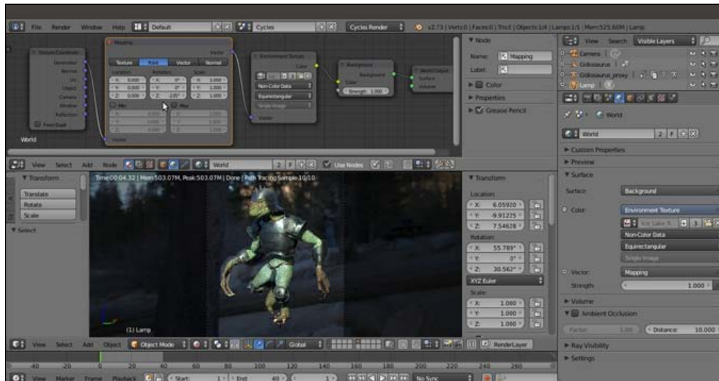
Rotating the hdr image to match the position of the Lamp
