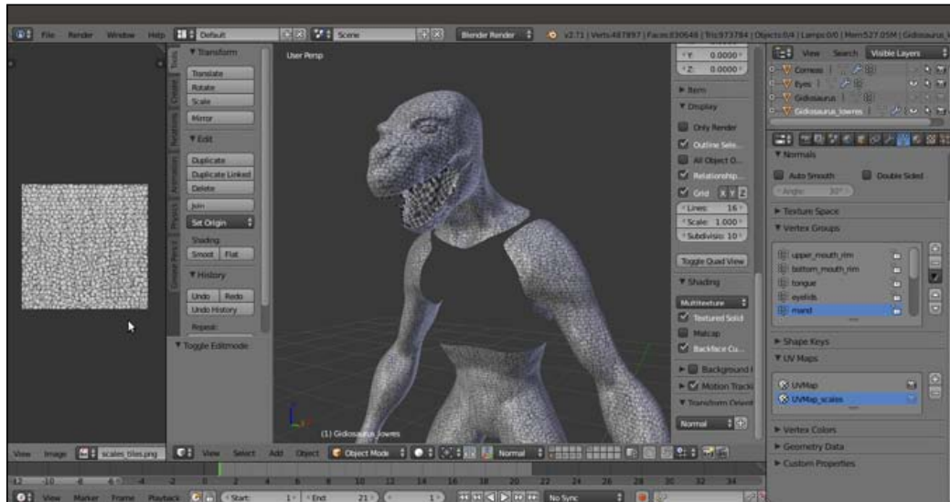
The scales_tiles.png image mapped on the model using the second UV coordinates layer
