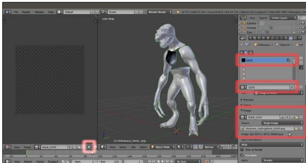
The assigned blank image loaded in the UV/Image Editor window and pinned to be displayed regardless of the object selection
