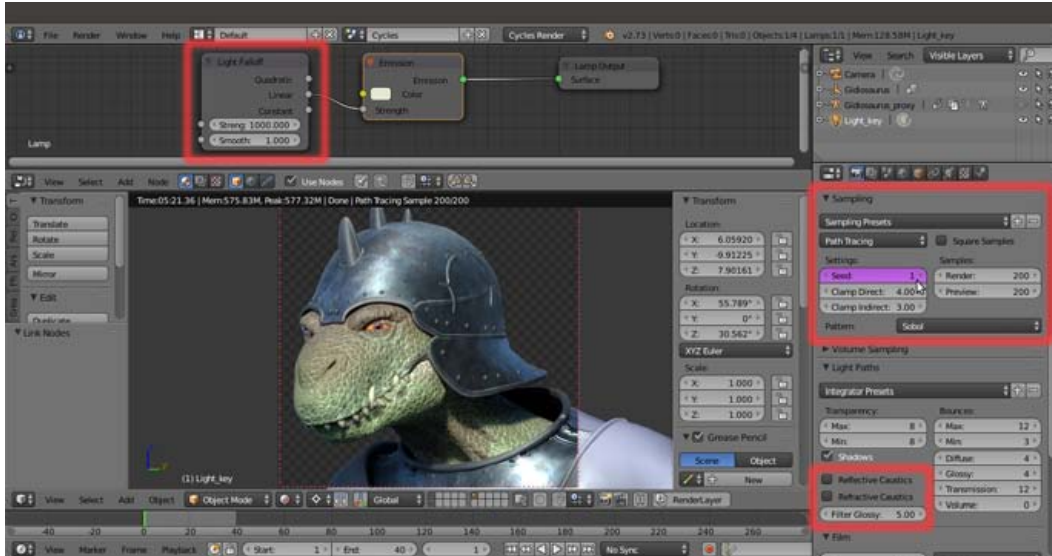
The Light Falloff node for the Lamps, the Seed driver for the noise, the Caustics items and the Filter Glossy value
