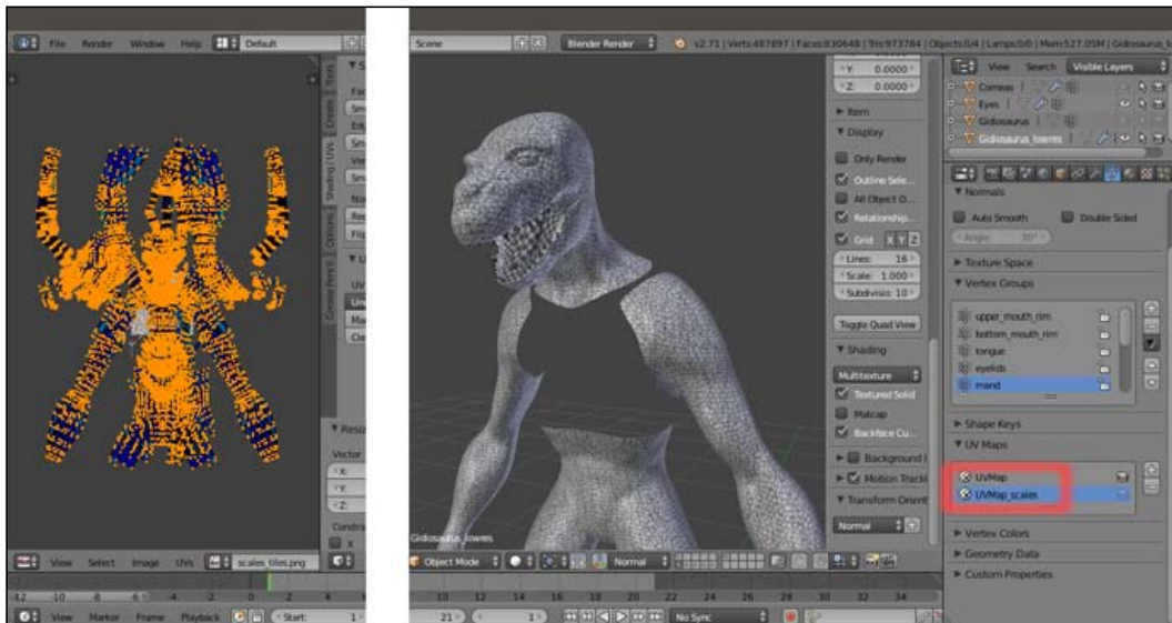
The two UV coordinates layers in the UV Maps subpanel
