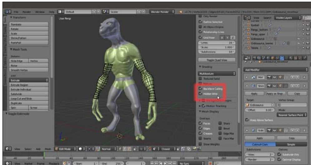
The second wireframe visualization method
