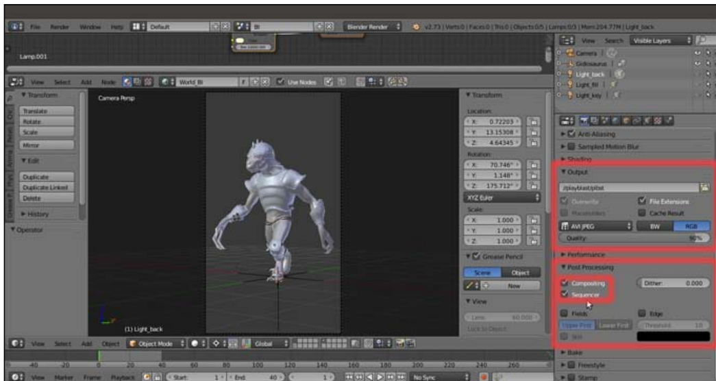
The Output and the Post Processing subpanels inside the Render window
