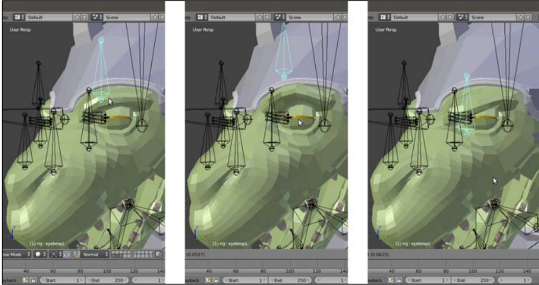
The same bone moving in two opposite directions to drive two opposite shape keys
