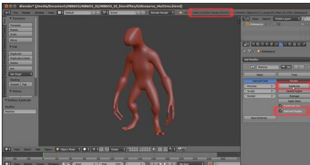
The mesh with a Multiresolution modifier assigned at level 3 of subdivision
