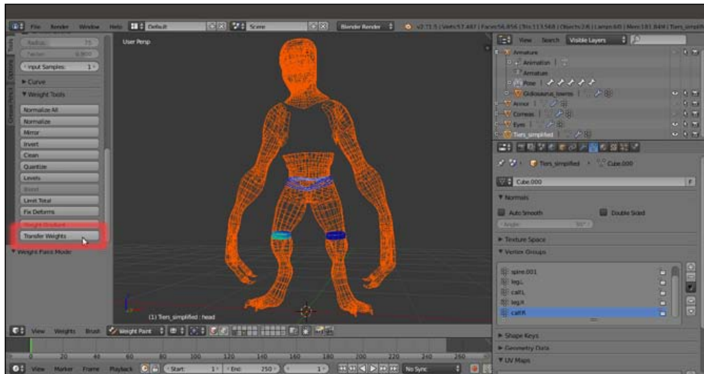
Transferring the vertex group weights from the Gidiosaurus mesh to the tiers object
