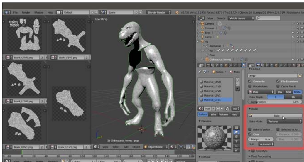
The 5 baked images and the Bake subpanel under the Render window
