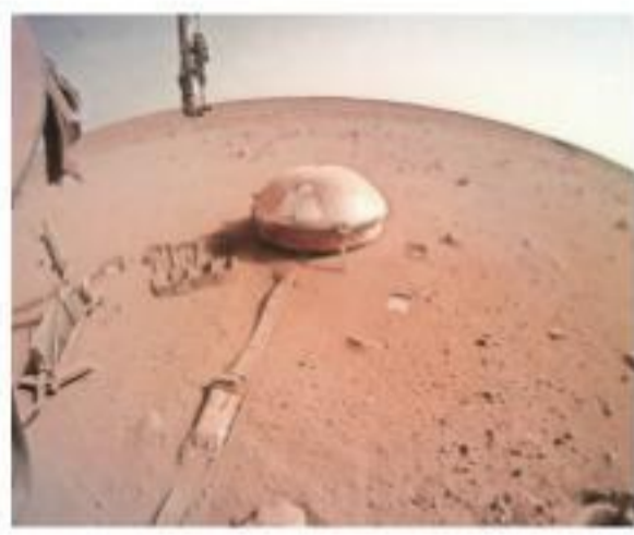
The dome-covered seismometer belonging to NASA's InSight lander, on Mars. NASA/JPL-Caltech
