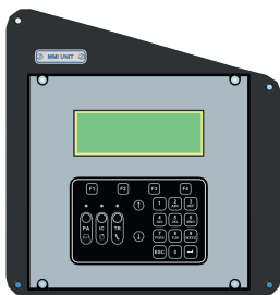
Fig 4.11 Panel-9_ MMI unit of PIS (Operation by Assistant Driver)
