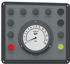
Fig 4.10 Panel-8_ Cabin Control Switches for Assistant Driver and Gauges
