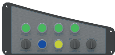
Fig 4.12 Panel-10_ Doors Control Switches
