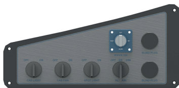
Fig 4.3 Panel-1_Cabin control Switches
