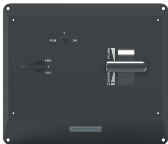
Fig 4.15 Panel-12_ Master Controller & indication switches
