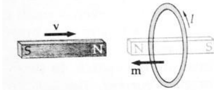
Doing work on a magnet to create a current is the basis behind an **electrical generator**. In hydroelectric dams, falling water turns large paddles connected to electrical generators that convert mechanical energy to electrical energy. Conversely, we can use changing flux to **do** work. This is the principle behind an electric motor.
