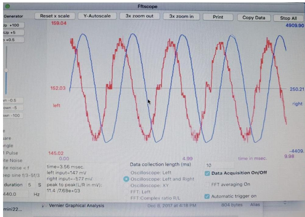
You will now induce an emf in the smaller coil using a changing magnetic field supplied by the outer coils. There will be no motion of the coils involved. The signal generator will provide the outer coils with a fluctuating current to vary the magnetic field, and hence the magnetic flux, through the inner coils. The fluctuating current will be sinusoidal, triangular or square in waveform shape.
