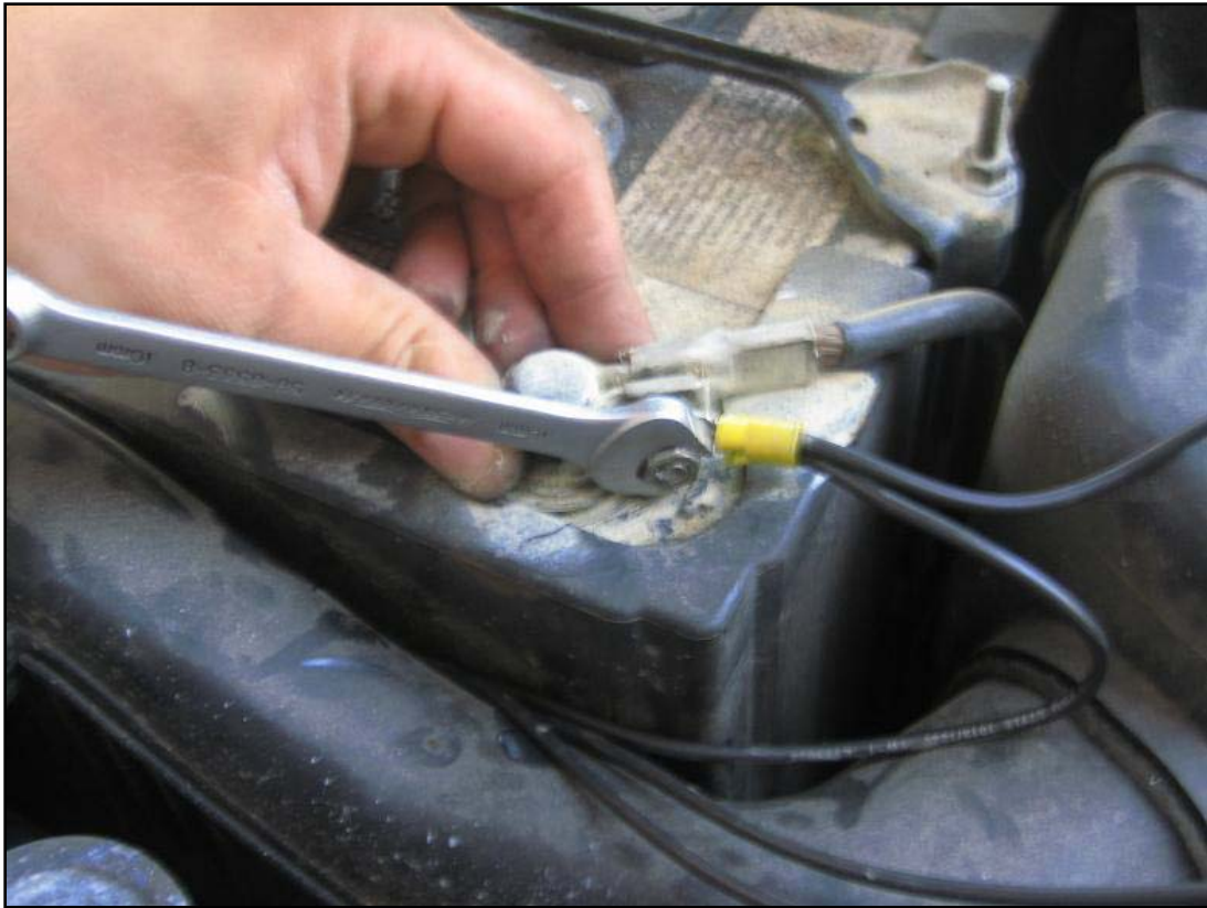
Splice Connector only for the Trigger Wire. #86 on Relay
