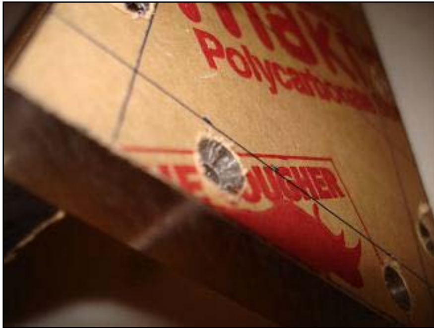
Indicator lines shown with holes drilled and countersunk
