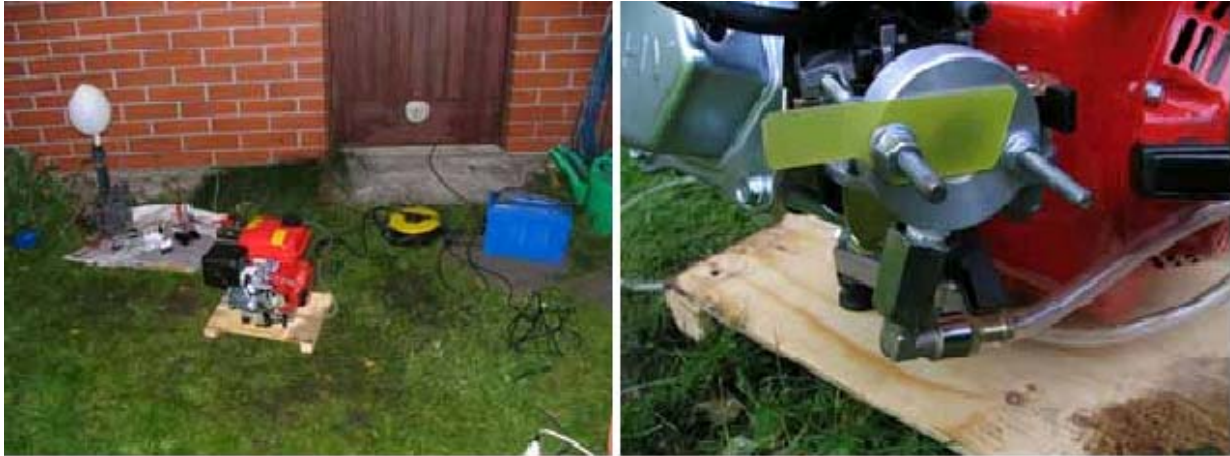
Figure 14. 6.5hp 200cc 4-stroke running on electrolytic gas
