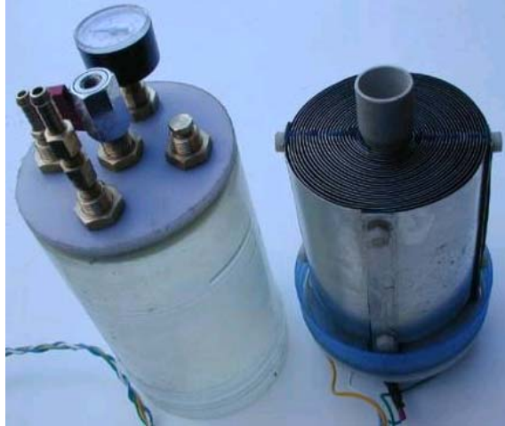
AntDavison 's spiral electrolyzer based on the Shigeta Hasebe_design
